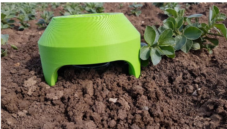
Figure 10. Raised cover over pitfall trap to prevent rainfall inundation.
