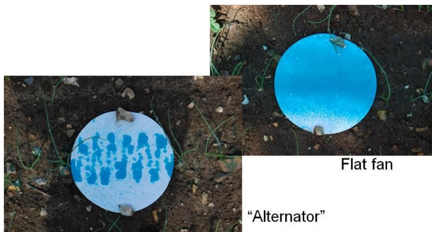
Figure 21. Deposits on the horizontal collectors sprayed with the two nozzles used in the study
