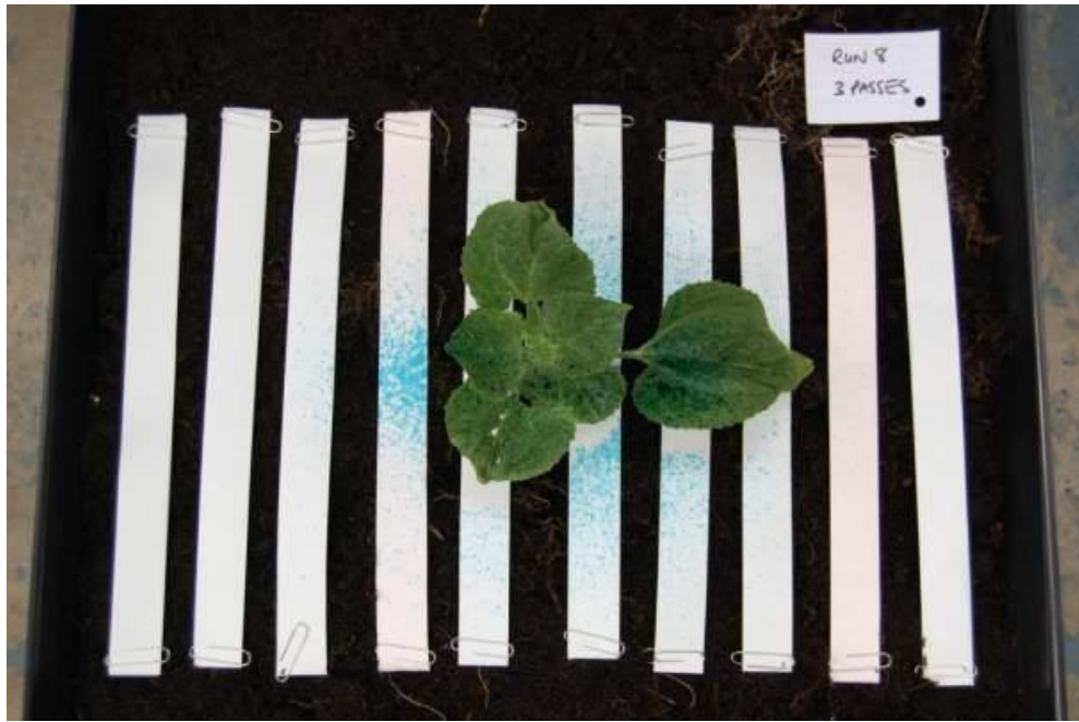
Figure 13. Dye deposits monitored on a plant surface treated with the “Even-Spray” nozzle operating 400 mm above the target, at a pressure of 3.0 bar and travelling at a speed of 4.0 km/h in still air conditions. (Note: The larger footprint compared with the “Alternator” nozzle and little evidence of secondary splash from treated leaves).
