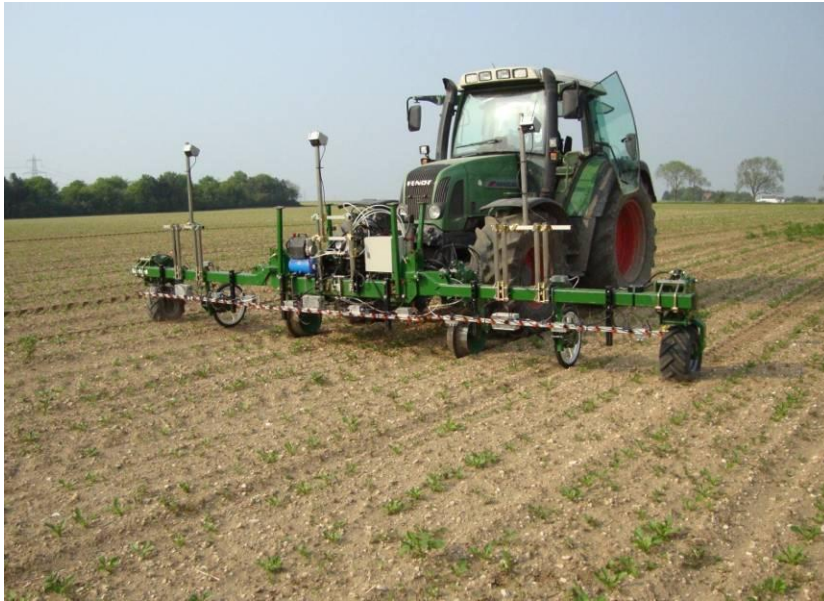
Figure 42. Experimental machine operating to spot spray volunteer potatoes in the sugar beet crop in May 2012.
