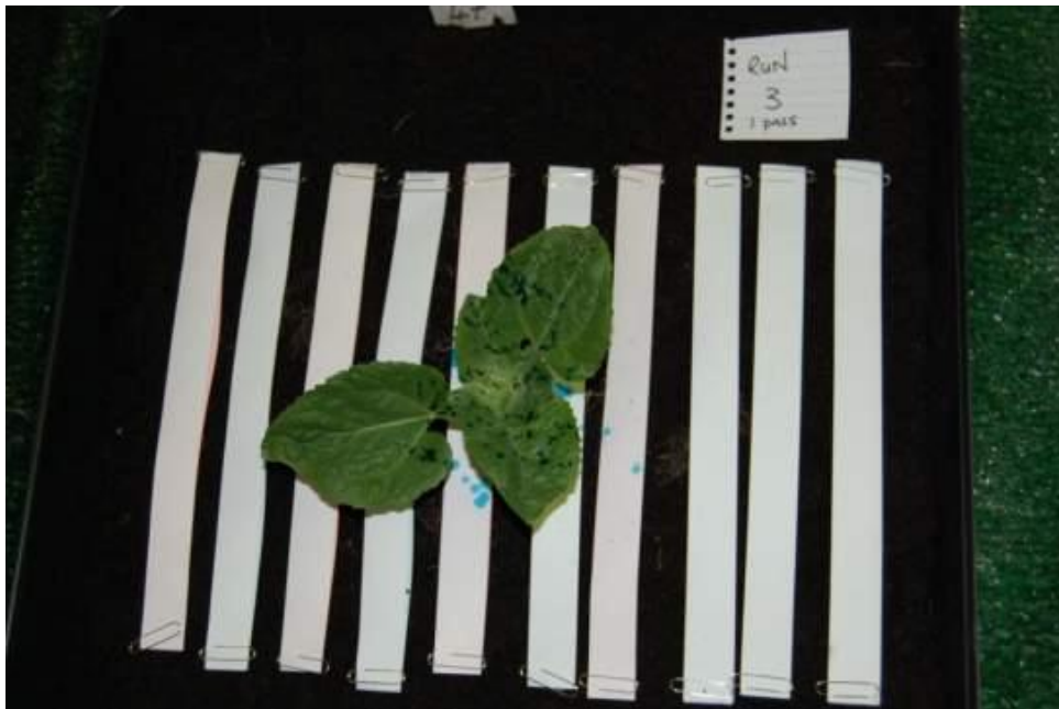
Figure 12. Dye deposits monitored on a plant surface treated with the “Alternator” nozzle operating 400 mm above the target, at a pressure of 0.75 bar and travelling at a speed of 4.0 km/h in still air conditions. (Note: Little evidence of secondary splash from treated leaves).
