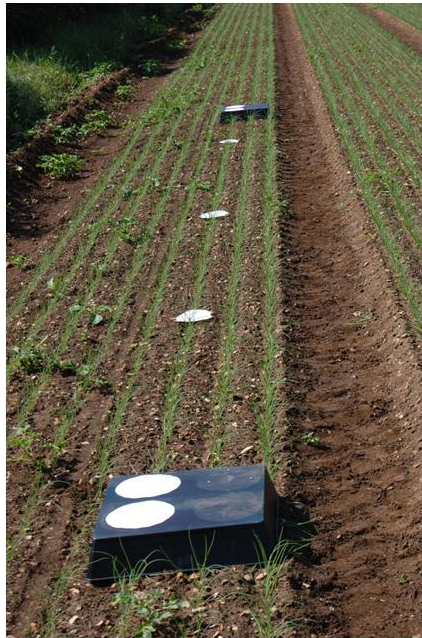
Figure 20. Experimental layout for sampling deposits on horizontal surfaces and onion plants in field conditions
