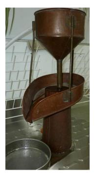
**Picture 3:** Modified Fenwick Can Cyst washer used to separate the organic matter fraction of soils.
