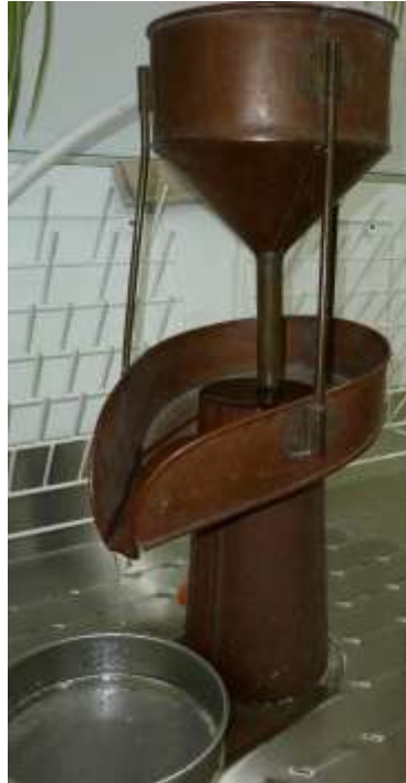
Figure 2 The Modified Fenwick Can used to separate out the organic matter content of the soil.
