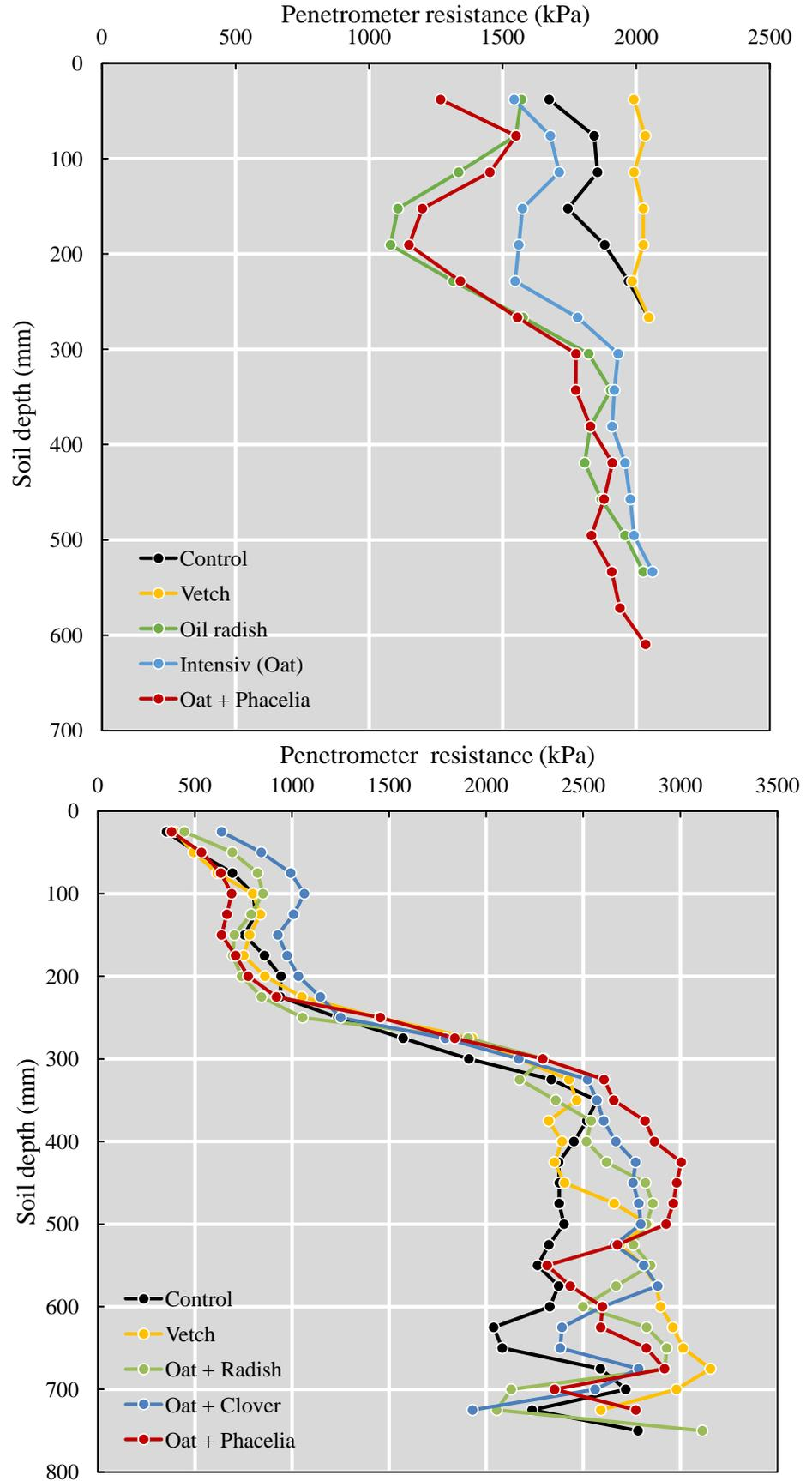
**Figure 12:** Soil penetrometer resistance profiles. Boxtree Bubwith (top) showing lesser compaction after certain cover crop mixes (June 2017). Vicarage FS (bottom) after heavy rainfall, plough pan obvious at 250-300mm (June 2019).
